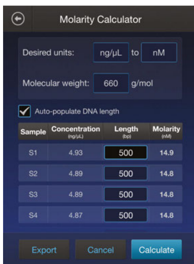
Figure 7. Molarity Calculator. Use the Molarity Calculator to quickly convert the length of nucleic acid and concentration to molarity.
